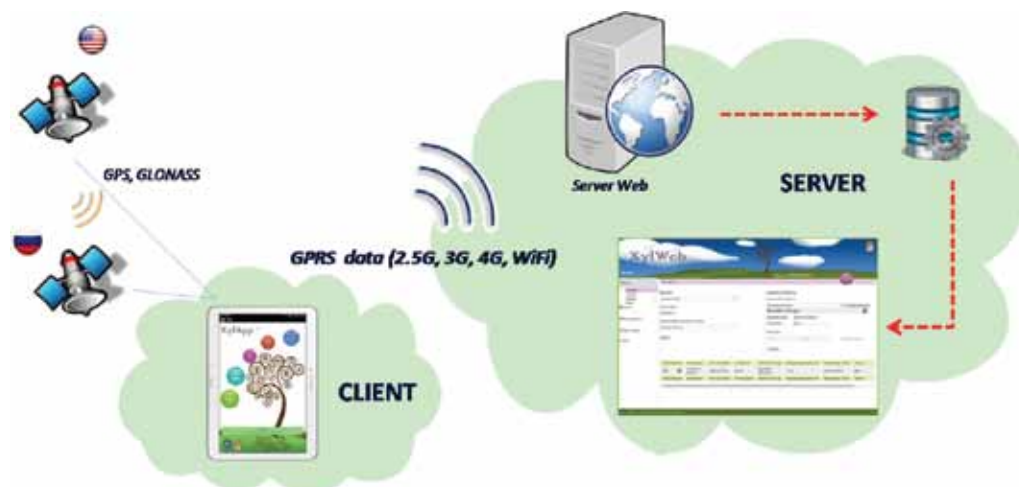
Figure 1. Client server architecture: XylApp - XylWeb.
