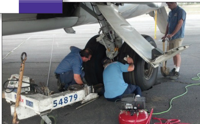
Right: Maintenance personnel examine a disabled B727 aircraft at KRAL airport in Riverside, CA. The aircraft, too heavy for the general aviation airport's ramp design, unexpectedly sank into the asphalt during a pushback procedure.
