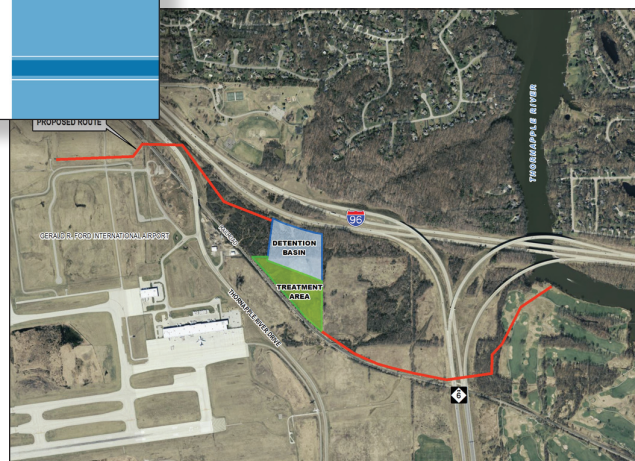
Right: Proposed route for redirected stormwater flows at Gerald R. Ford International Airport. The route utilizes twelve natural treatment beds.
