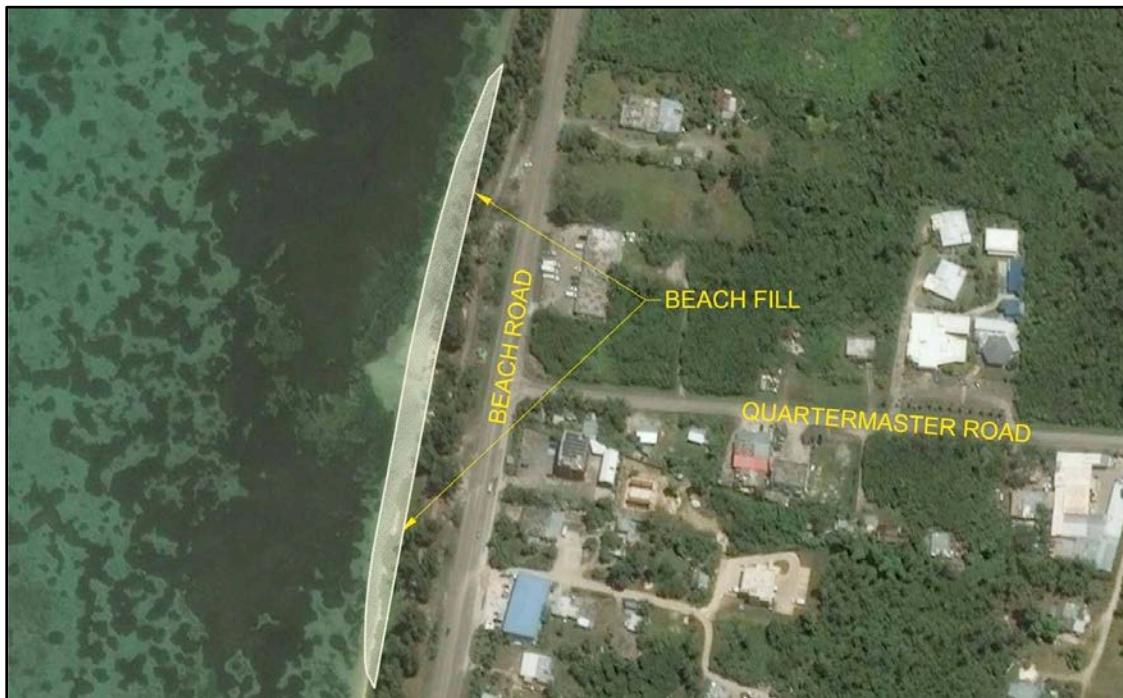
Figure 36. Beach nourishment project footprint with a length of 1,000 feet and a 70-foot seaward extension of the shoreline that could be accomplished with approximately 28,000 cubic yards of beach quality sand.
