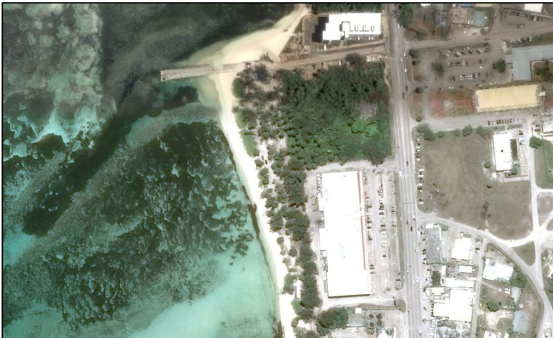
Figure 32. Accretionary fillet that has formed to the south of Sugar Dock due to its interception of northerly directed littoral drift.
