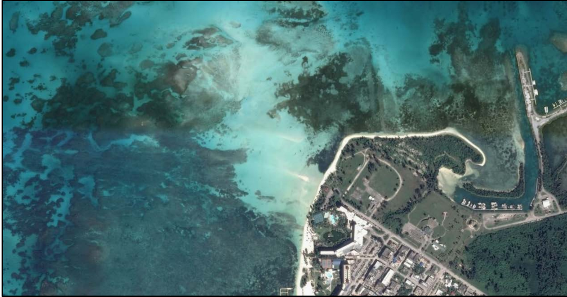
Figure 33. A sandbar has formed offshore of AMP's western shoreline that could be a potential sand source for beach nourishment.
