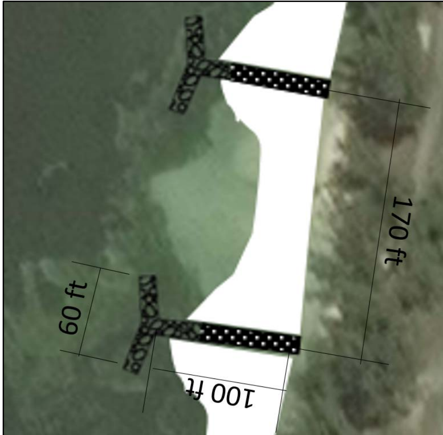
Figure 38. Approximate dimensions of the T-head groins shown in Figure 37 (spacing 170 feet, stem length 100 feet and head width 60 feet).
