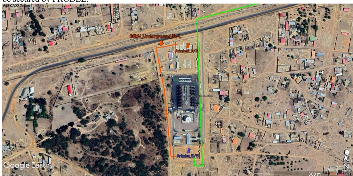
Figure 7.4-1 Route Diagram of 60 kV Underground Distribution Line
