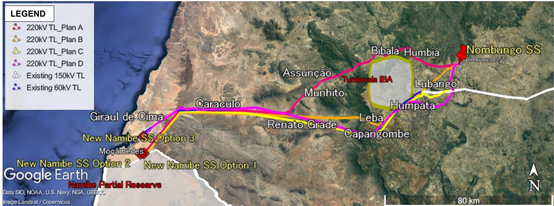
Figure 9.4-1 Project Area and Alternative Transmission Line Routes
