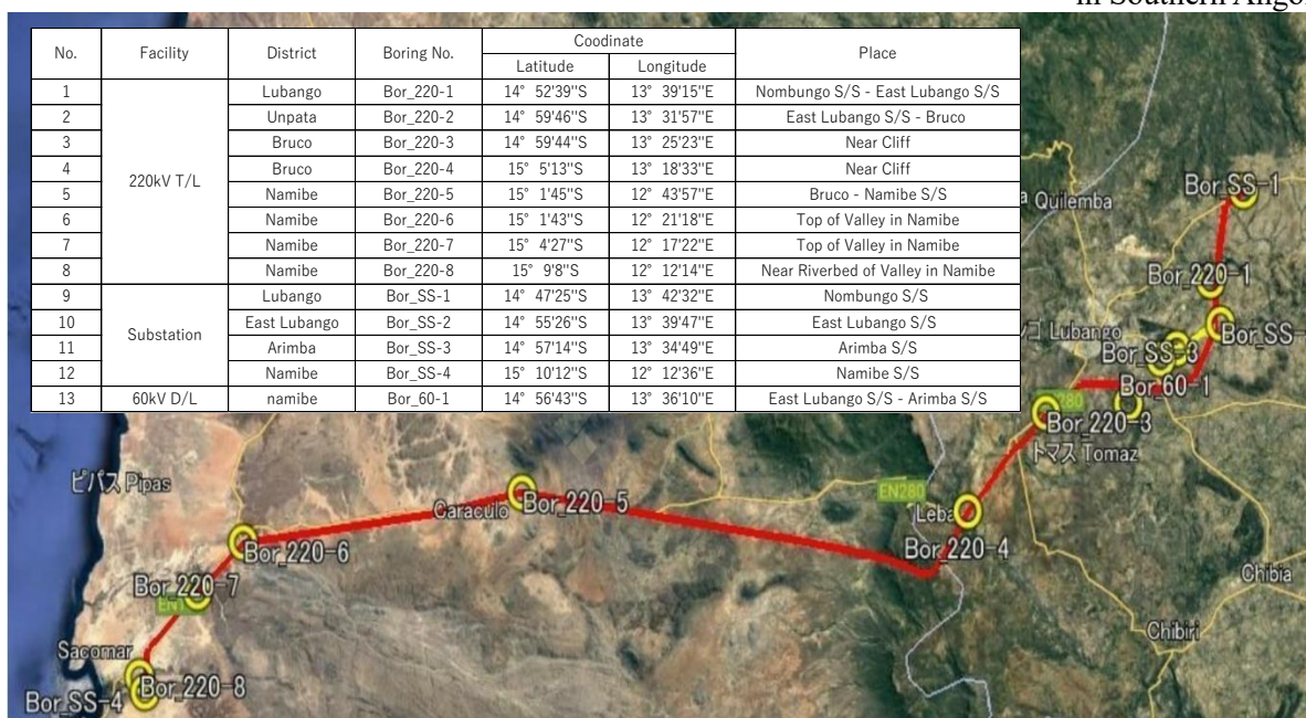
Figure 5.3-1 Geological Survey Boring Locations
