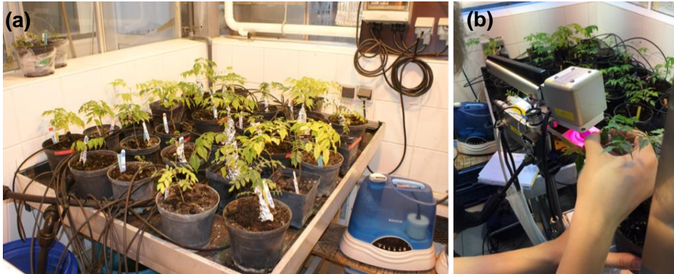
Figure 5.1 Controlled experiment on 1-year old potted E. ivorens and E. suaveolens seedlings (a) and leaf gas exchanges measurements with the Licor system (b, Li-6400, Licor, Inc., Lincoln, NE, USA)
