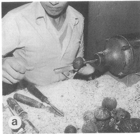
10. a, The ivory nut is placed on the lathe and b, carved into the foot of a salt shaker. Colombia, Dept. of Boyaca, Chiquinquirá.
