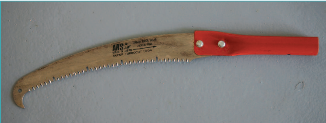
2. The saw head and mount cuts on the back-stroke and has sawdust-removing gullets.
