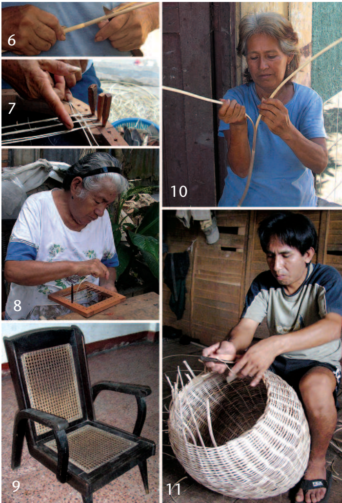
6–11. Manufacturing and some products of vara casha ( Desmoncus polyacanthos ) in Iquitos, Peru. 6. Splitting of fresh stem. 7. Chair seat with each cross skein cut to measure and fastened by glue. 8. A weaver, 75 years old. 9. Armchair with seat woven of vara casha ; part of a 25–30 years old living room suite. 10. Splitting of stem into halves. 11. A weaver using half stem skeins with pith to produce a basket; a labor of about two hours.
