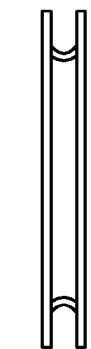
Capillary tube. Meniscus at each end is pinned to inner wall. Evaporation occurs at ends but not center resulting in radial flow.
