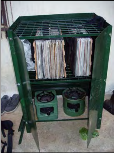
Figure 10. Field dryer using kerosene stoves as a heat source.
