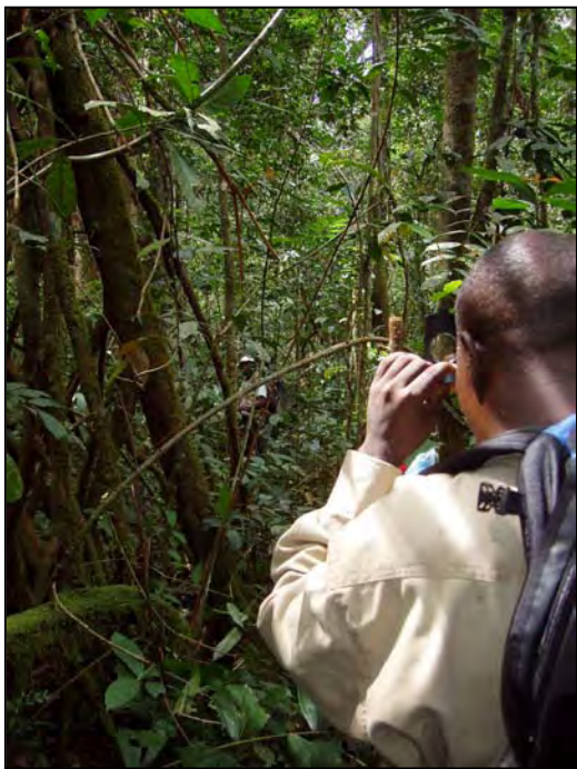
Figure 4: Line sighting using a compass
