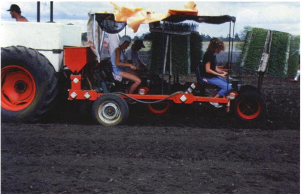
Plate 7 A four-row planter adds fertiliser and water to the seedlings as they are planted (R.Colton)
