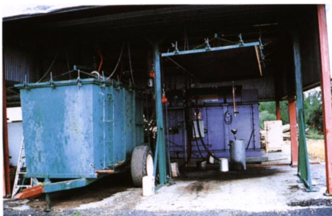
Plate 17 Two-pot distillery with boiler and separator in the background, sealed mobile bin (left) and suspended bin lid (right) (R.Colton)
