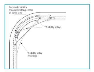
Figure 10.1 - Measurement of forward visibility
