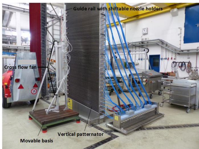
Figure 2: Experimental set-up in front of the vertical patterner.
