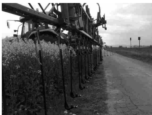
Figure 1: Sprayer with dropleg nozzles
