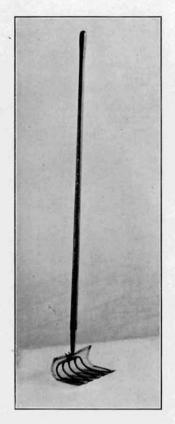
b. Potato hook with prongs covered with wire netting, for removing mud from ditches.
