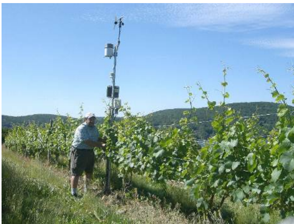
Dr. Ferrandino checking sensor connections for a weather station deployed within a Chardonnay vineyard located in New Preston, CT.
