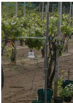
Rotorod unit deployed in vineyard to catch powdery mildew spores. DNA extracted from spores of the powdery mildew fungus is amplified using PCR and produces a distinct molecular band (red arrow) after electrophoresis.
