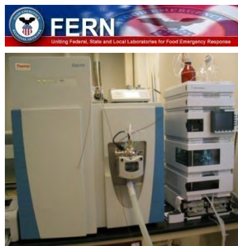
Figure 2. The Exactive LC-MS calculates molecular mass to four decimal places and enables accurate determination of violative pesticide residues and toxins in food.
