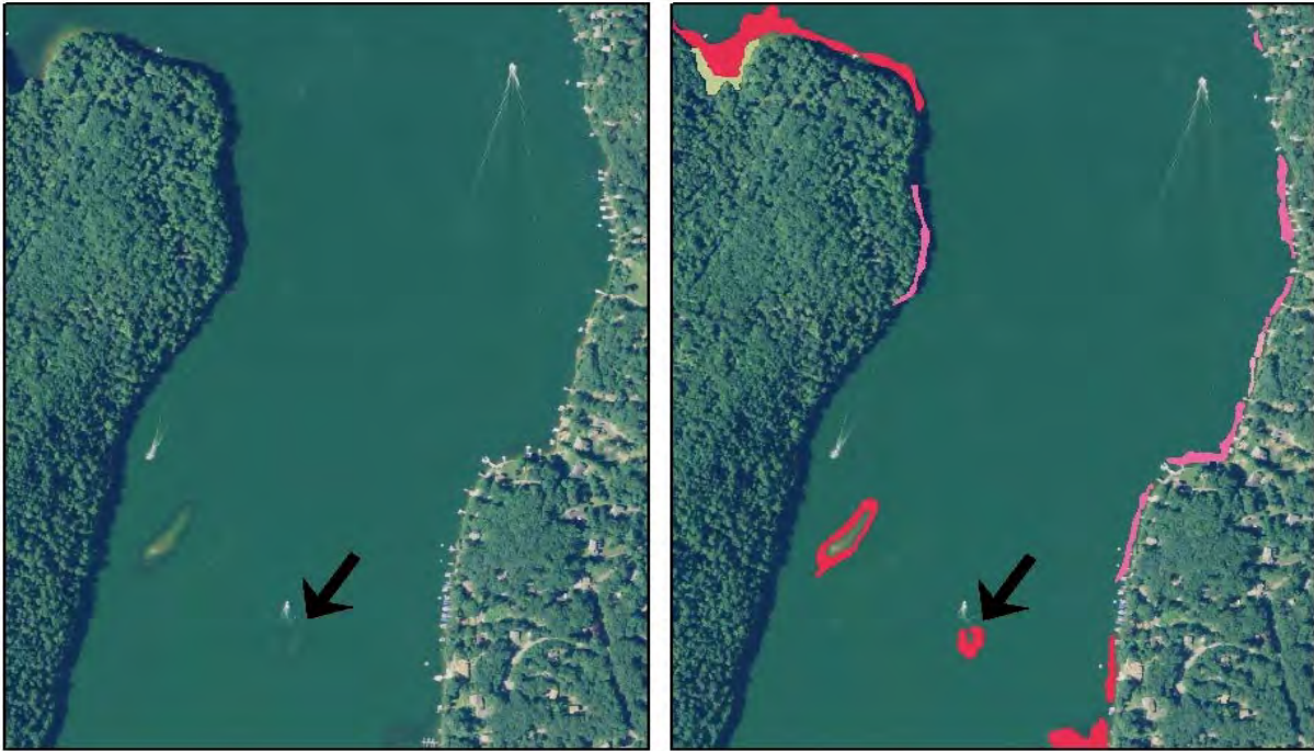
Figure 2. Remote sensing imagery suggested area (arrow left) was M. spicatum . This was confirmed by our field survey and an invasive polygon was added to map (arrow right). The other polygons (right) were found without remote sensing but their visibility in the imagery is striking.
