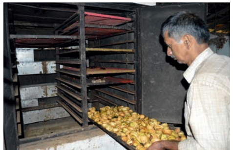
Plate 72 Improved energy-efficient fruit rind dryer
