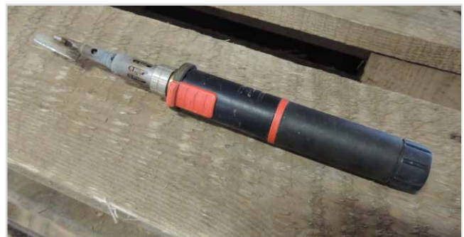
6. Hot knife used for pruning and harvesting. The knife operates on liquid gas and can be refilled as easily as a cigarette lighter
