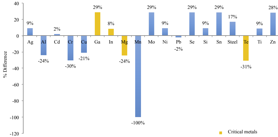
Fig. 9. Change in metal inventory according to forecast market share of PV modules.
