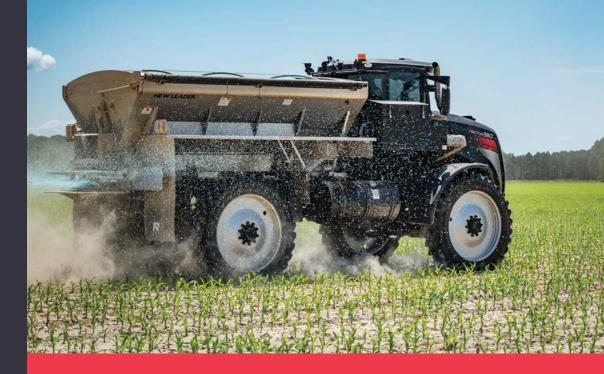
PRESSURE COMPENSATED HYDRAULICS HELP MAINTAIN RATES, EVEN AT LOW ENGINE RPMS.
