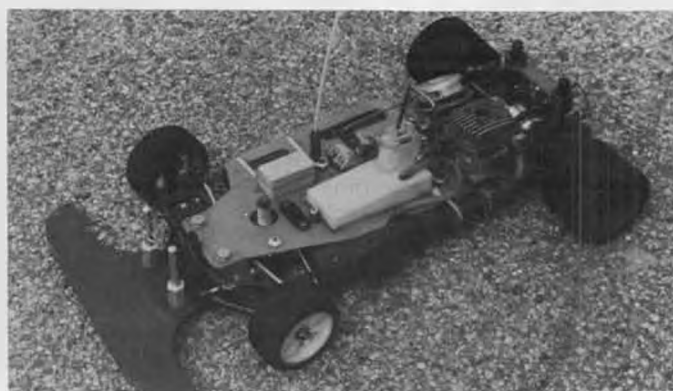
The Booth-Preston prototype car for Associated. Front end parts ahead of kingpin axis for more room.
