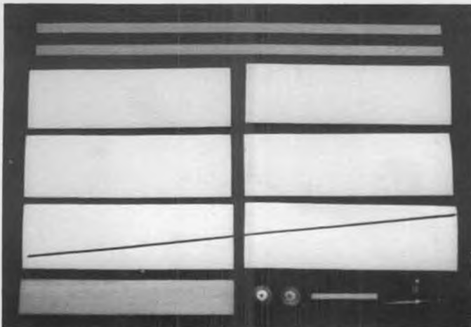
Masic materials; foam wings, balsa sticks, 1/8 wire (on lower wing set in photo), wheels, 1/2A engine, some 1/8 balsa, and scrap wood.
