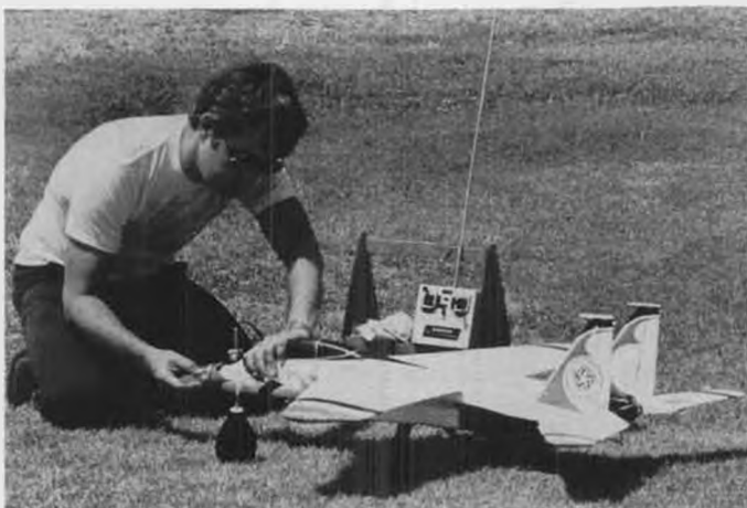
Author likes the simple things; squeeze bulb fueler and hand starting. F-15 R.O.G.s despite long grass.
