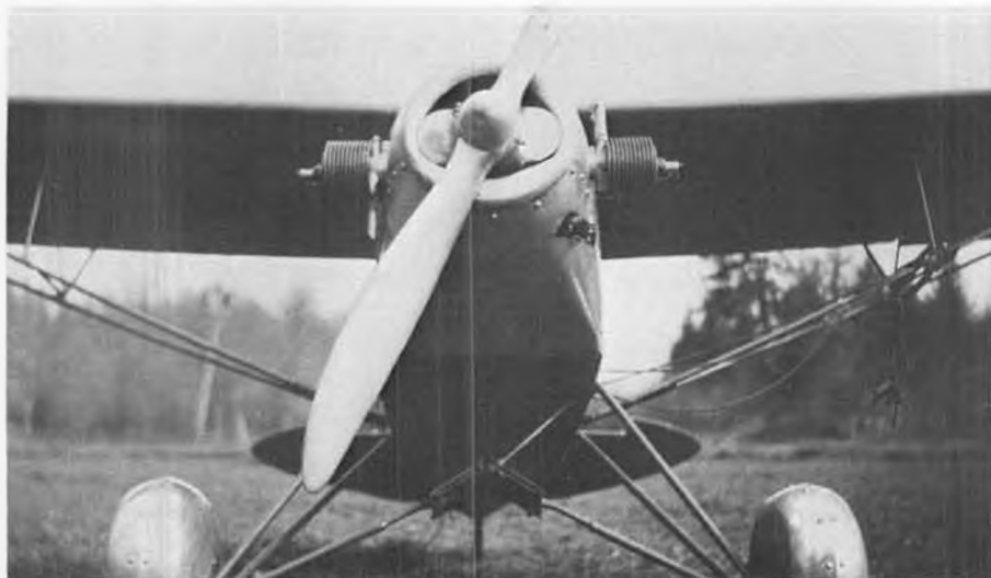
Front end of the first control line model. Twin Forster 99's turned prop clockwise through auto oil pump gears.
