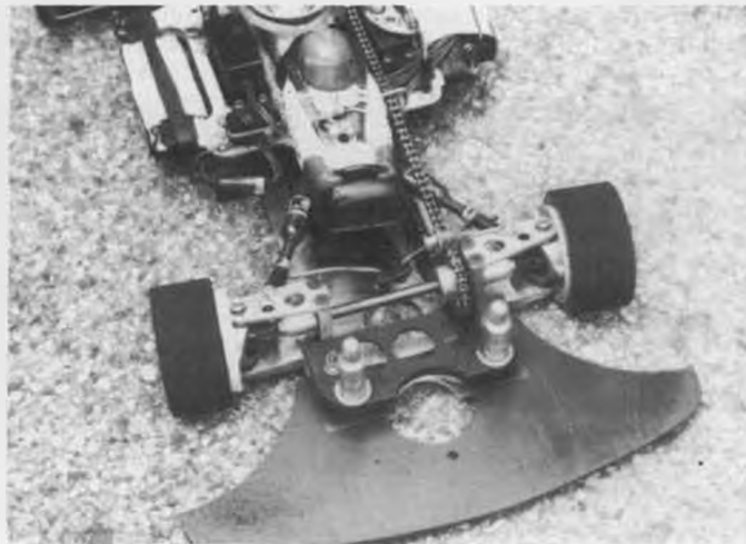
Taki added new front end and chain drive components from Kyosho off-road car. Aluminum cylinders are one-way clutches.
