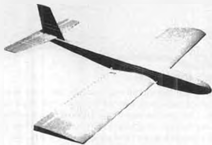
"RIDGE RAT" - $44.95 49" span Slope Sailplane Area - 436 sq. in., Wt. - 32 oz. Wing Loading - 10.6 oz/sq. ft.
