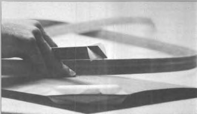
One-inch wide laminate strip on a 12-inch wide sheet. Protective scrim cloth is peeled back.
