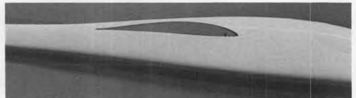
Fit-up of wing fairing using "cast-in-place" technique explained in text.
