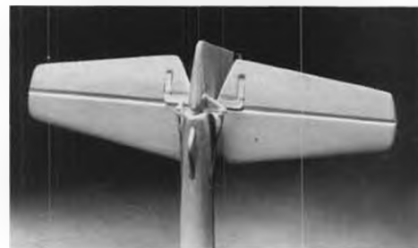
Flies with 2-channel radio for rudder and elevator control.
