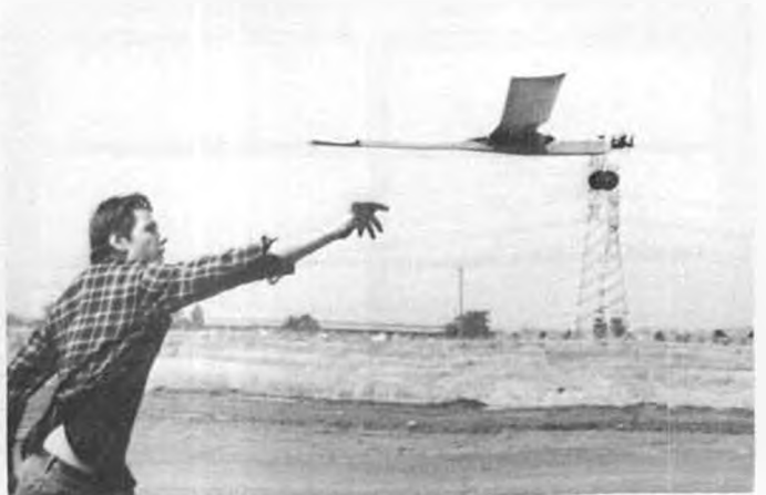
Launching model for test flight. Note that it is in a level attitude.
