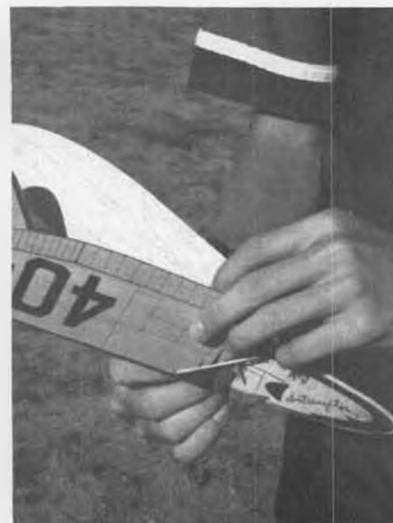
Steps in launching the Interceptor. Hold fuselage under wing. Lift up trailing edge of wing with fingers of other hand. While holding wire support, fold wing back along fuselage.
