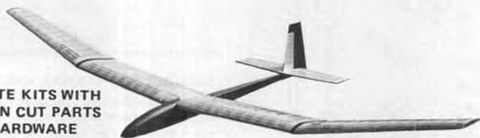
"PARAGON" - $79.95 118" span Thermal Soarer Area - 1080 sq. in., Wt. - 48 oz. Wing Loading - 6.3 oz/sq. ft.
