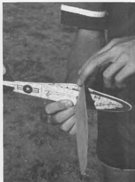
Steps in launching the Interceptor. Hold fuselage under wing. Lift up trailing edge of wing with fingers of other hand. While holding wire support, fold wing back along fuselage.
