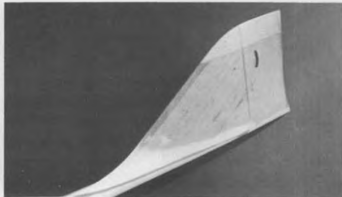
Fin attached and fillet completed. K&B primer used as final contouring aid/filler on fin, fillet, and fuselage.
