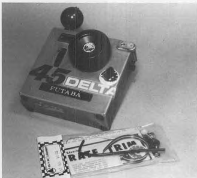
Update kits from Delta, to add adjustable steering rate to existing transmitters. An easy installation.
