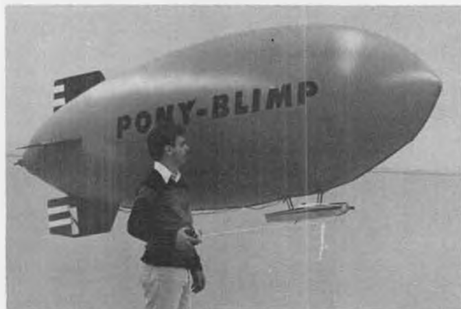
The Pony-Blimp by Peck-Polymers. Length 11 feet, diameter 4 feet, uses three to five-channel radios.
