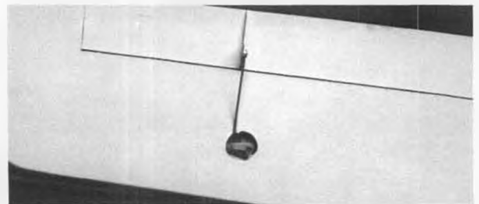
Aileron bellcrank access. Geometry is different from that shown on drawing.
