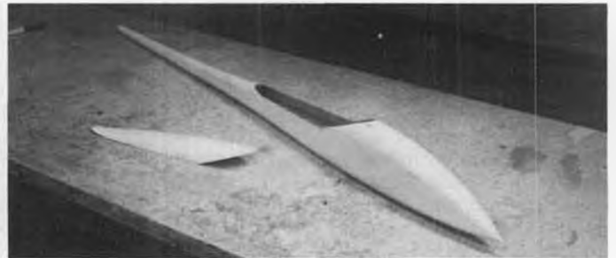
Foam has been removed and hatch cut free. Allow to air out for a day or so.
