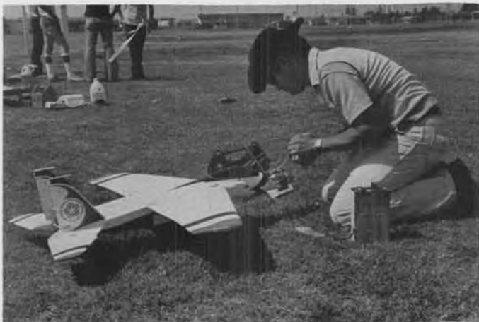
Generous tailplane areas assure smooth, responsive sport flying. Horizontal tail is full-flying stabilator.
