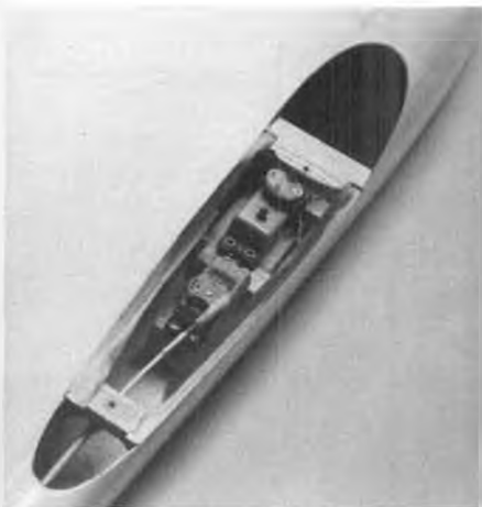
Servo installation. Note Kavan pushrod to elevator servo, aileron coupling ball on servo output disc. Disc stiffened with epoxy circuit board. Old wing mount. Follow plans.
