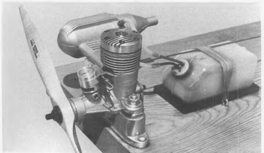
The M&H Variable Venturi Carburetor installed on MB's K&B 61 for testing purposes. Note: no hole in the top of the carb!
