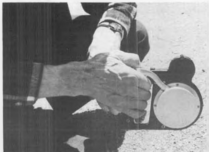
With this modified "U-Reely" handle, Oba can perform flat spins. It automatically takes up line slack.
