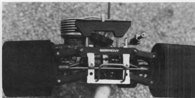
Rear hub pivots on Serpent OK, but if car lowered with suspension deflected, geometry would be better.
