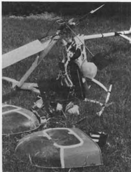
Somehow this doesn't look as neat as the original kit! Vibration detuned the receiver.
