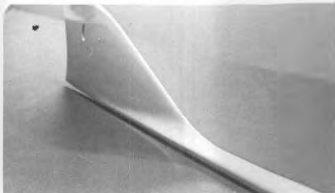
Final finish of fillet gives smooth, flowing lines, minimum drag.
