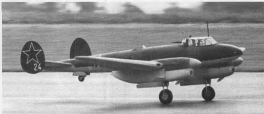
John Preston catches Bob Underwood's 2nd Place PE-2 on takeoff. Two HP .40's, 12-3/4 lbs., flaps, retracts, dive brakes, bomb drop, stainless steel kitchen sink, etc.
