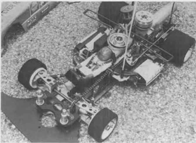
The 4 wd Kyosho prototype car. Same component layout as Kondo except muffler. Note three chain idlers.
