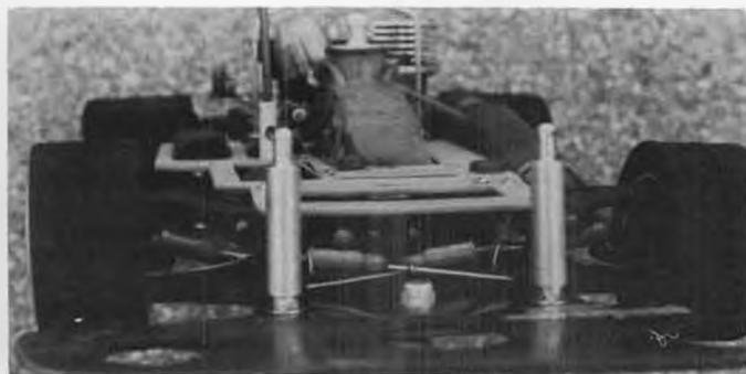
Serpent front suspension geometry pretty good, but top 'A' arm too steep. Front wires (with loop) are roll bar.
