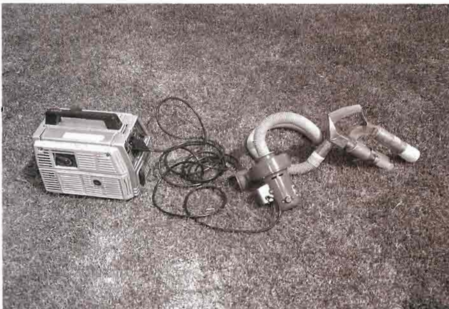
Figure 9. The components of a typical cyclone collector.
