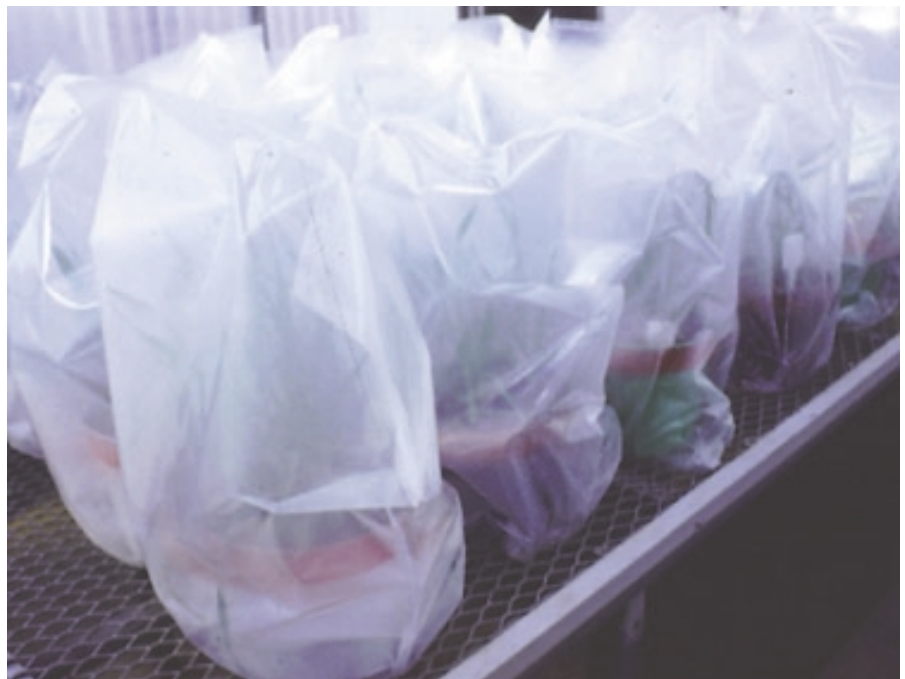
Figure 1.7. Ultrasonic humidifier modified to supply a cool mist of water in a plastic incubation chamber.
