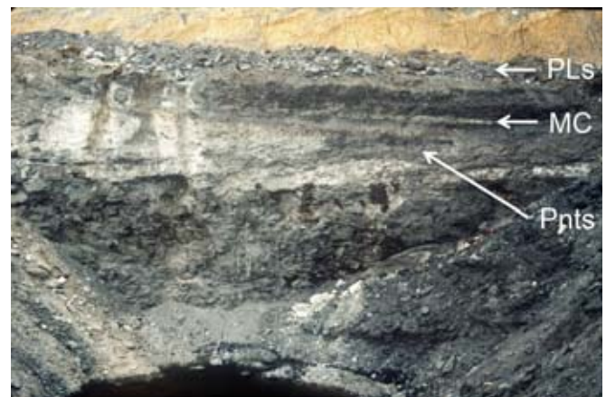
Figure 4. Stratigraphic section below the Perth Limestone (PLs) and above the Upper Block Coal Member (base of section, at waterline). Plant fossils (Pnts) were derived from below the Minshall Coal Member (MC) and its underclay in shales immediately above a series of en echelon sand bodies. Brazil Coal and Clay, Saline Pit No. 1, in 1988.
