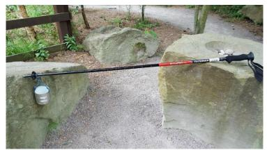
Figure 13. Water sampling device allowing easy and safe access to water courses.
