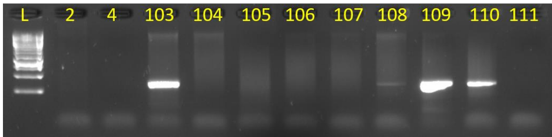
Figure 46: Gel electrophoresis result of P. guttata specific primer Pg2. L: 1kb Ladder, NTC: No template, expected amplicon size 375bp.
