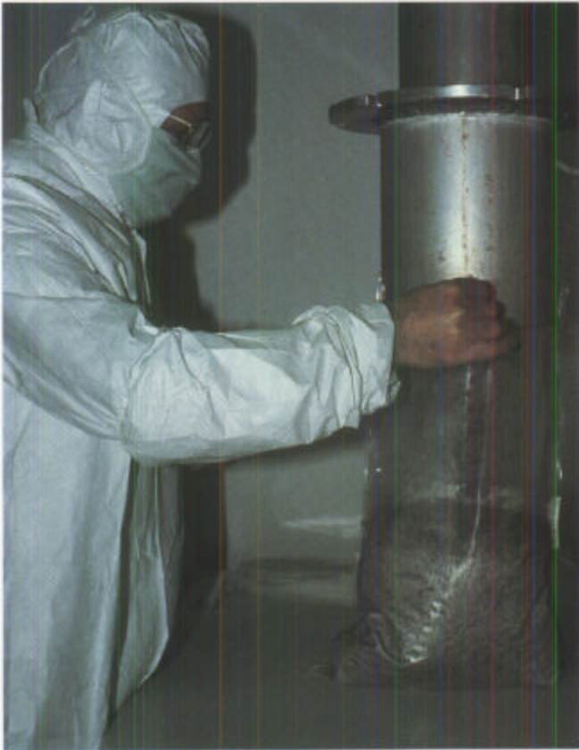
Figure 5.2.55 —Filling bags with vegetative inoculum in a peat-vermiculite carrier under aseptic conditions (courtesy S. Maul, Mycorr Tech, Pittsburgh, PA).
