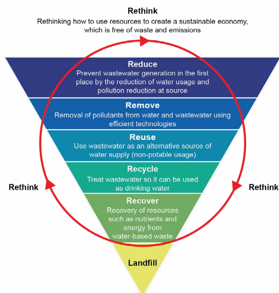
Figure 1. Circular economy model framework in the water and wastewater sector (based on Smol et al. , 2022).
