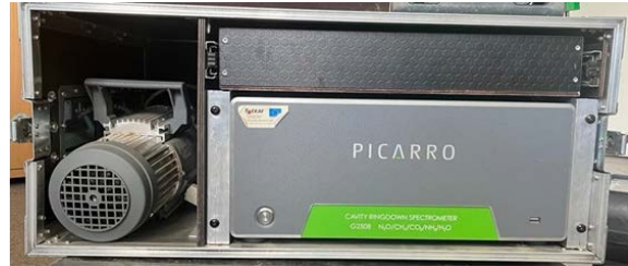
Figure 6. CRDS gas measurement device Picarro G2508 (Picarro Inc., USA California) with a vacuum pump. This combination enables the measurement process.
