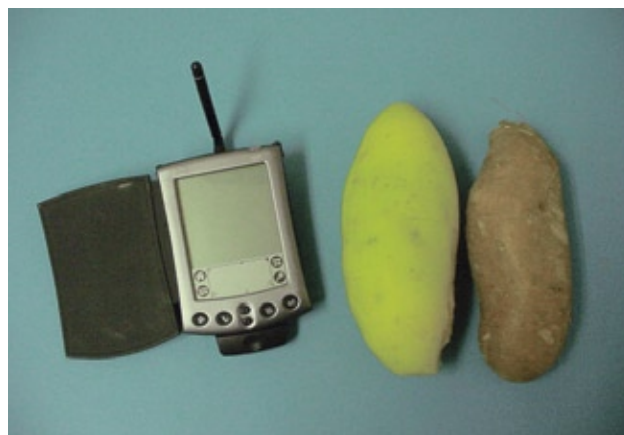
Figure 17. Instrumented impact recording device used to measure impacts on packing lines. Right: fresh sweetpotato; middle: molded urethane casing with accelerometer inside; left: handheld computer with antenna for receiving signal from accelerometer and recording impacts. (PHOTO BY B. EDMUNDS)
