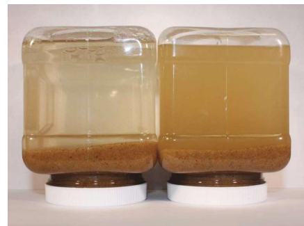
Shown are samples of DustPRO treated sand (left) vs. uncoated sand in water. (Source: Preferred Sands)
