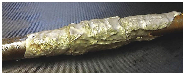
This GRE liner survived years longer than the oilfield tubular it was installed in. (Source: Duoline Technologies)
