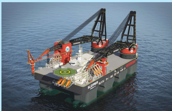
HMC's dual-fuel Sleipnir semisubmersible unit will be the largest crane vessel in the world, with two Huisman revolving cranes each capable of lifting 10,000 metric tonnes. (Source: Heerema Marine Contractors)
