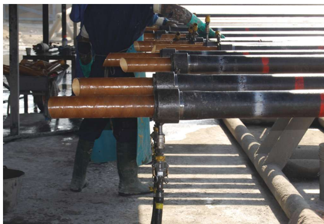
These GRE liners are being installed in oilfield tubulars. (Source: Duoline Technologies)
