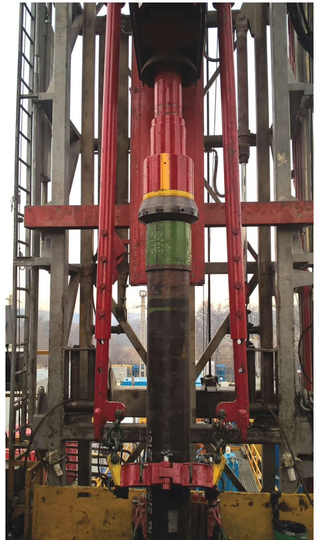
OMV Petrom has drilled more than 43 well sections using the Weatherford nonretrievable DwC system and Defyer casing bit. (Source: Weatherford)
