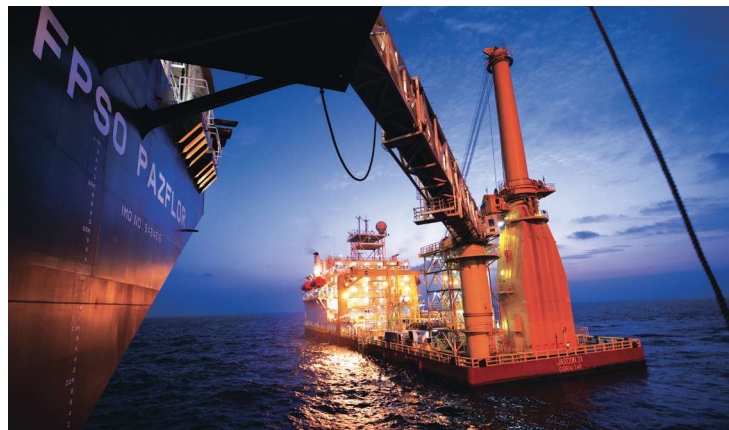
Total's deepwater FPSO Pazflor unit in Block 17 offshore Angola is bridge-linked to the Jascon 31 accommodation and construction vessel. (Source: Total)
