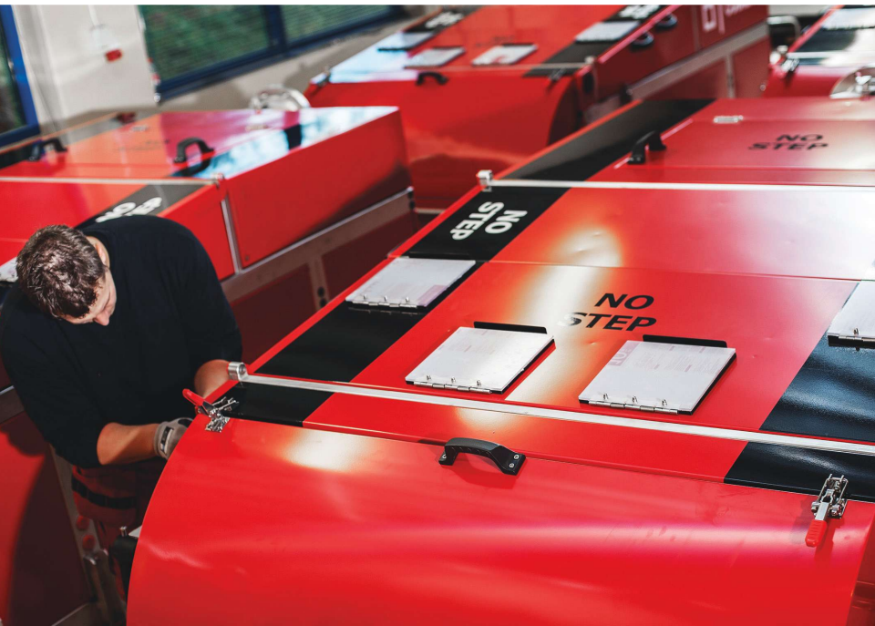
Drilling fluids are vacuumed through a rotating filter belt using high airflow to separate the cuttings from the fluid more effectively. The MudCube is a compact solids control system that eliminates using high levels of vibration to separate fluids and solids. (Source: Cubility)
