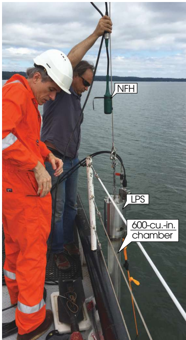
FIGURE 1. The LPS prototype is shown being deployed in Seneca Lake. A 600-cu.-in. firing chamber is hanging vertically below the main housing of the source. Above the source, there is a green NFH. Below the source already in the water (on an orange nylon rope), there is a vertical array of 24 FFHs. (Source: Dolphin Geophysical)
