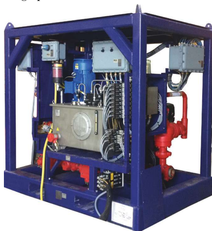
The HoD manifold, connected to the rig mud circuit, acts to divert flow from the standpipe line to the clamp and then to the valve, ensuring uninterrupted mud circulation when the top drive is disconnected. (Source: Drillmec)
