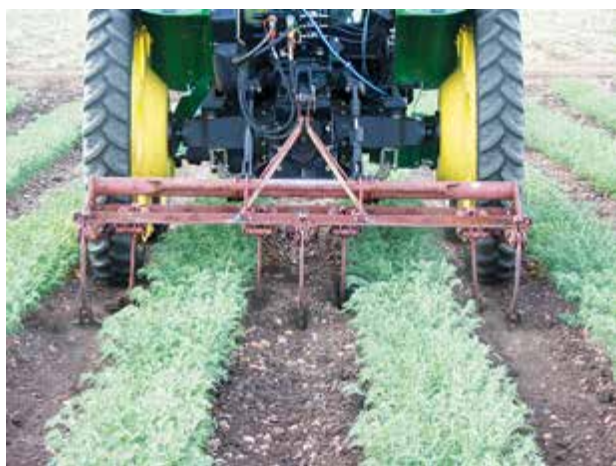
Figure T2.3b–1 Inter-row cultivation can be effective for controlling small and stressed weeds.
