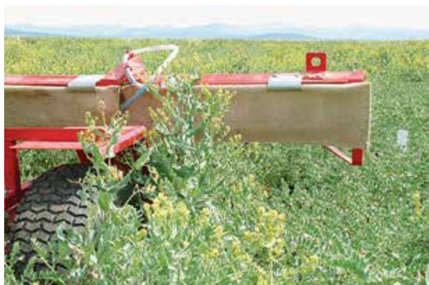
Figure T3.1c–1 Blanket wipers use a sheet (blanket) moistened with herbicide to apply to weeds above the crop.
