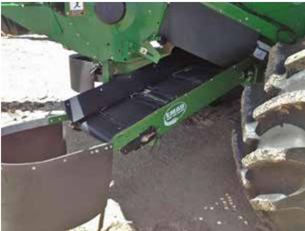
Figure T4.1e-5 Chaff decks use a conveyor to move the chaff and weed seeds onto the wheel tracks in a controlled traffic farming system. Photo: Warwick Holding
