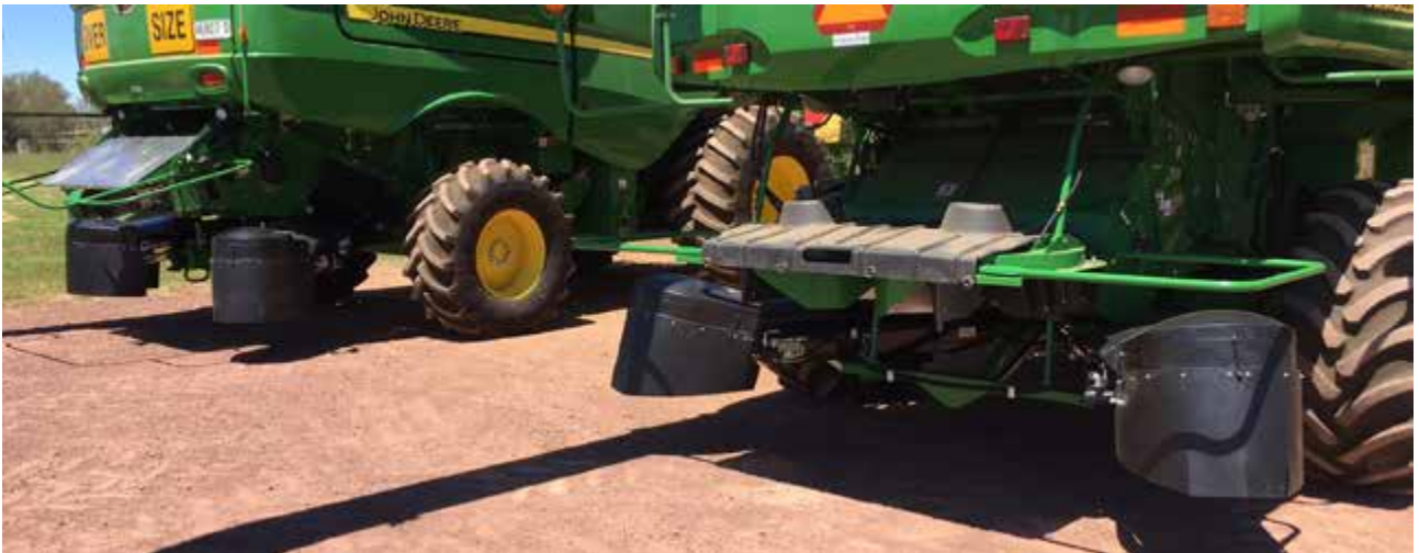
Figure T4.1e-4 Chaff decks used in a controlled traffic farming system. Photo: Warwick Holding
