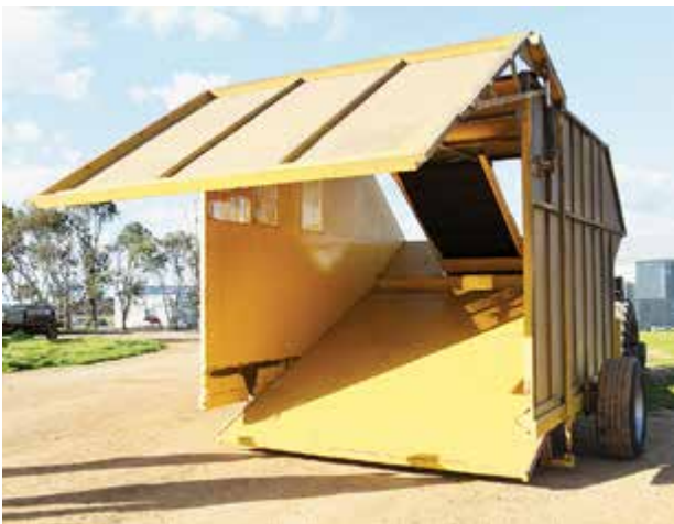
Figure T4.1b-4 Dumping system for large capacity chaff cart.
