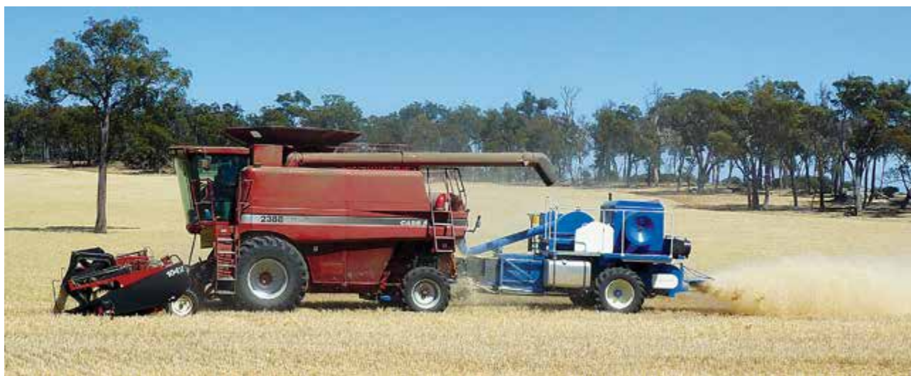
Figure T4.1d-1 Harrington Seed Destructor Mark III during the 2012 harvest.
