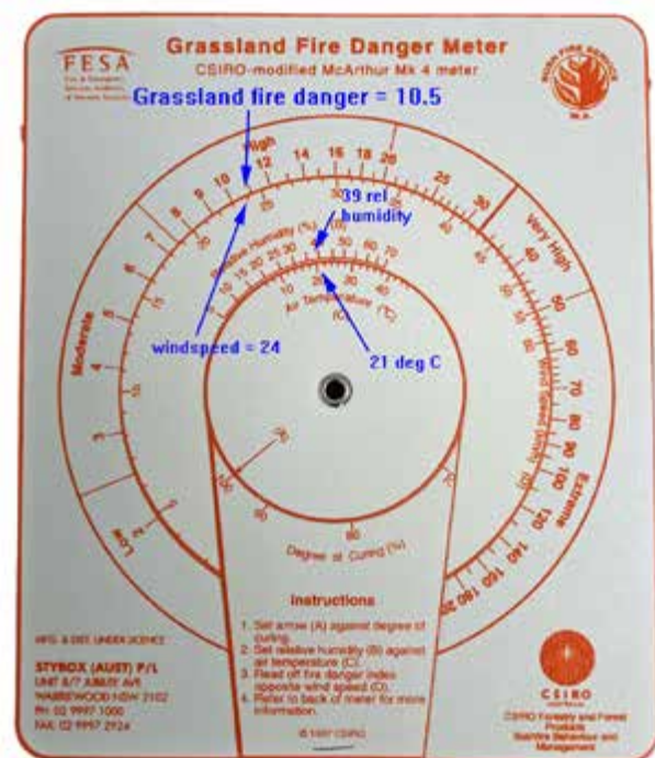
Figure T4.1a–3 The McArthur Grassland Fire Danger Meter that can be carried in the glove-box.
