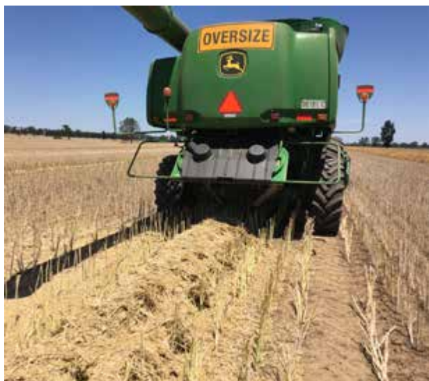
Figure T4.1e–1 Chaff chutes direct all material from off the sieves including weed seeds into a concentrated row.
