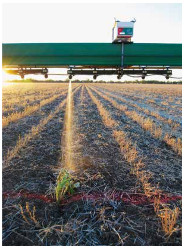
Figure T2.5–2 WEEDit weed detector sprayer applying herbicide to large spear thistle in a Victorian fallow.
