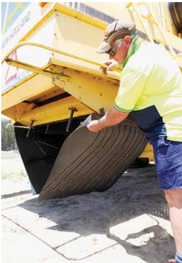
Figure T4.1–2 Doug Smith, Pingrup, WA, demonstrating how easy it is to build a shute to produce narrow windrows.
