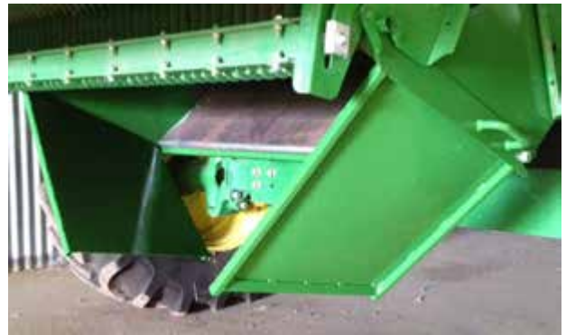
Figure T4.1e-6 Grower fabricated chaff chutes. Photo: Warwick Holding
