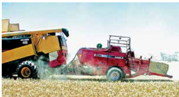
Figure T4.1c–1 Baling crop residue directly from the header minimises weed seed return to the seedbank.
