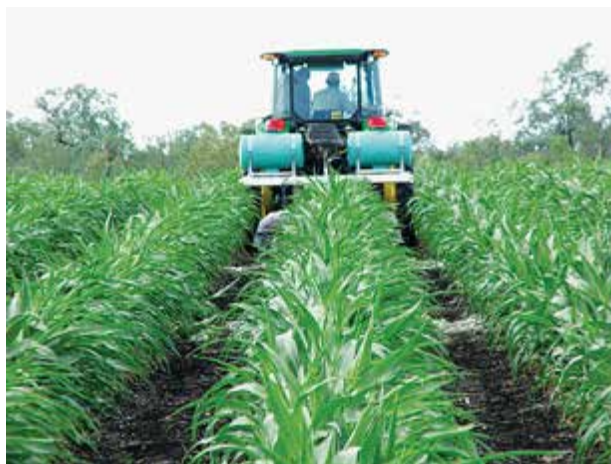
Figure T2.3–1 Inter-row shielded spraying in sorghum
