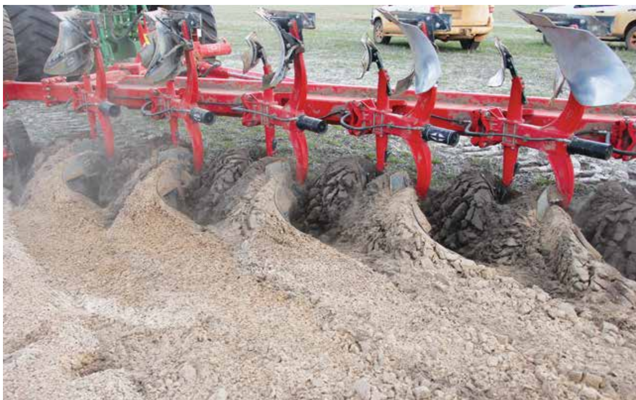
Figure T1.3–1 Mouldboard plough working near Geraldton showing skimmers in action.
