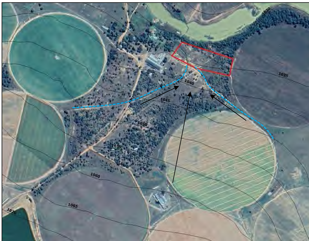
Figure 6-2-1 : Google Image showing the position of the stormwater diversion canals
