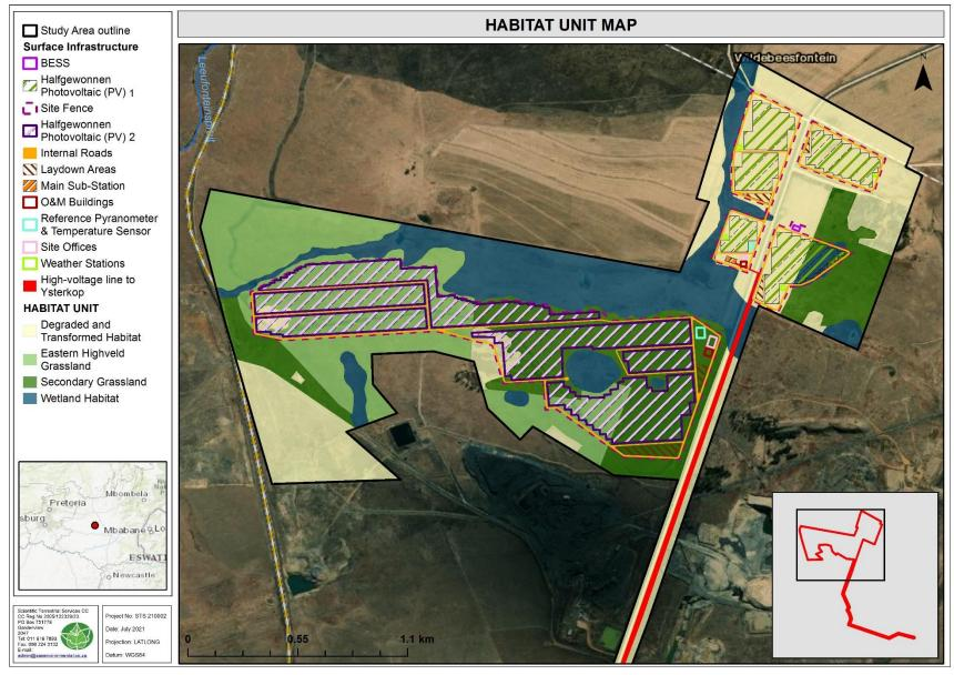
Figure 4: Conceptual illustration of the proposed surface infrastructure and linear developments (northern section of the study area) and their relation to the vegetation communities identified on site.
