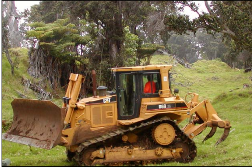
Figure 4. A D4 caterpillar with ripping attachment was used for the soil turnover treatment.
