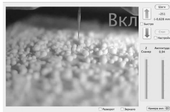
Figure 1. Microcapsules heat accumulating material SPM on the substrate (appearance)
