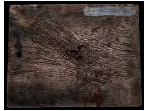
Fig 17 The metal master die for the 1½d. recess stamp re-engraved for 1925, and showing Harrison's indentations on the reverse
