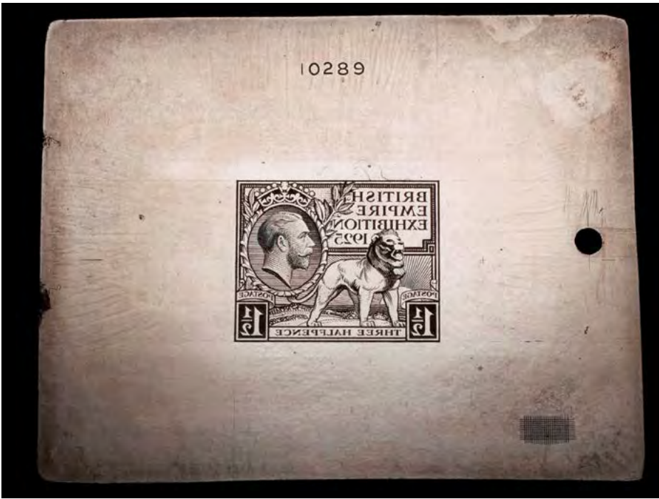
Fig 17 The metal master die for the 1½d. recess stamp re-engraved for 1925, and showing Harrison's indentations on the reverse
