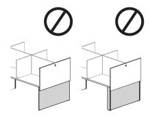
Carrel End Screens – Solid cannot be installed in combination with End Gable (THLBG) or Rectangular Base (THLBR)
