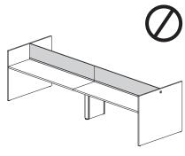
Is not designed to be installed in combination with Add-On or Add-On Framed Screens (THSAG, THSAS, THSFG, THSFF)
