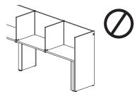
Cannot be installed in combination with another end support
