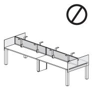
Is not designed to be installed in combination with Add-On or Add-On Framed Screens (THSAG, THSAS, THSFG, THSFF)
