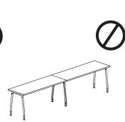
Worksurfaces with ADA Adaptable Legs Cannot be specified shared with 33" high ADA Adaptable Leg
