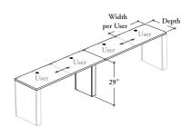
This table is recommanded for library and is available with or without divisions. It also is recommanded to be used againts a building wall for aesthetic.
