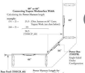
Power Harness Length for Connecting Trapeze Worksurface
