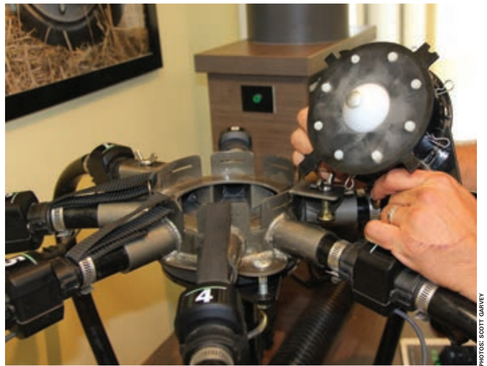
"Tuneable" distribution towers are a key feature made possible by adopting the new XeedSystem flow monitoring system.
