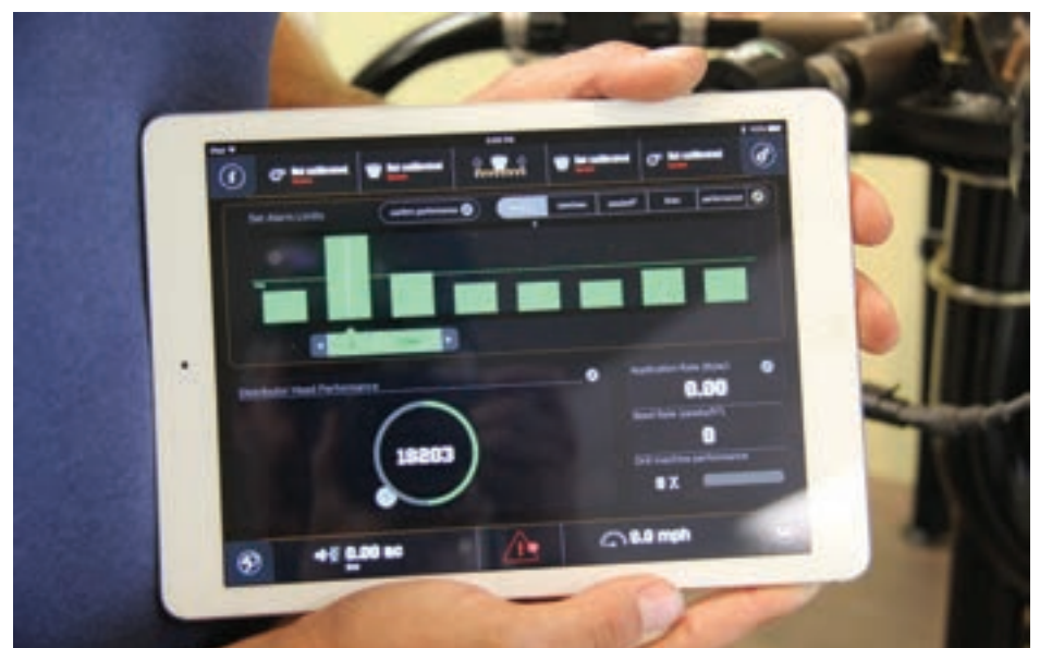
A monitor in the tractor cab keeps the operator updated on product flow and distribution.
