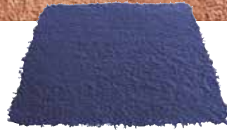
Veronica Stone (M) The design is similar Bush Stone, and appears to be created by a mason's bush hammer with a pitted and irregular surface.
