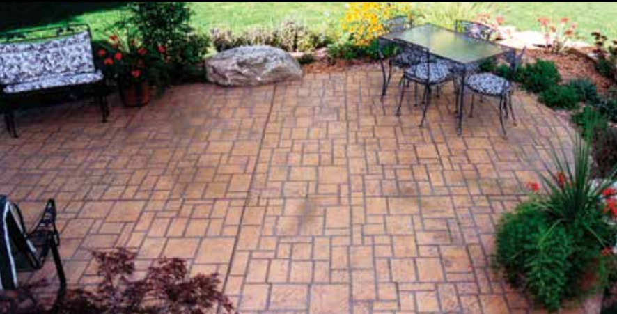
BUSHROCK AVERAGE STONE SIZE: 16" X 10" ROLL WIDTH: 36" JOINT WIDTH: 1/2"
