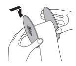
**5** Place the take-up reel into place behind the printer, above the roll paper.
