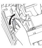
**3** Note the (+) and (–) markings in the battery compartment. Load a set of two new "AA" type alkaline batteries so that their plus (+) and minus (–) ends are facing as indicated by the markings.
