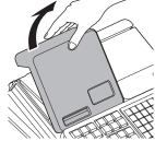
**2** Remove the battery compartment cover.
