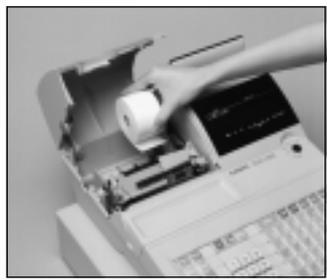
**4** Ensuring the paper is being fed from the bottom of the roll, lower the roll into the space behind the printer.
