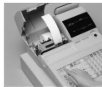
**6** Press the **JOURNAL FEED** key until about 20 cm to 30 cm of paper is fed from the printer.
