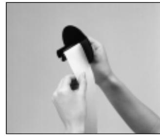
**7** Slide the leading end of the paper into the groove on the spindle of the take-up reel and wind it onto the reel two or three turns.
