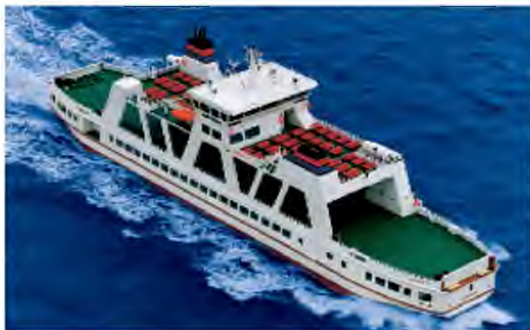
Figure 1: DEF FRISIA, 4 x VSP 16KG/100 - each VSP 470 kW input power, working in the North Sea in extreme shallow water
