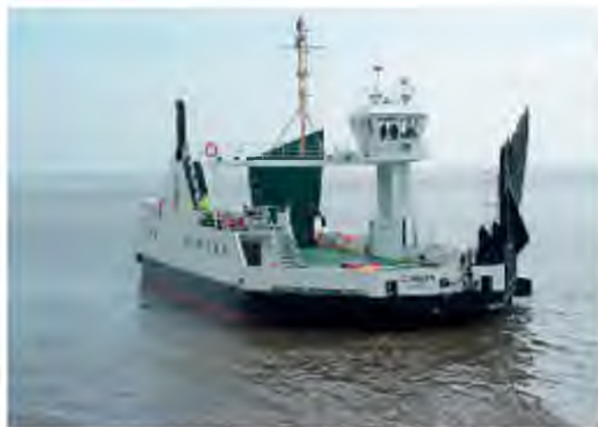
Figure 2: DEF CORRAN, 2 x VSP Gr. 16KG/100 - each VSP 470 kW input power, working in Scotland
