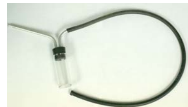
Figure 47. Aspirator for collecting melaleuca psyllids
