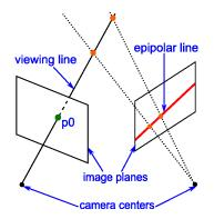
**Figure 2.11:** Epipolar geometry : if the projection of a 3D point is known to be p0 in a viewpoint, the projection in another viewpoint lies on the epipolar line of p0 (red line).
