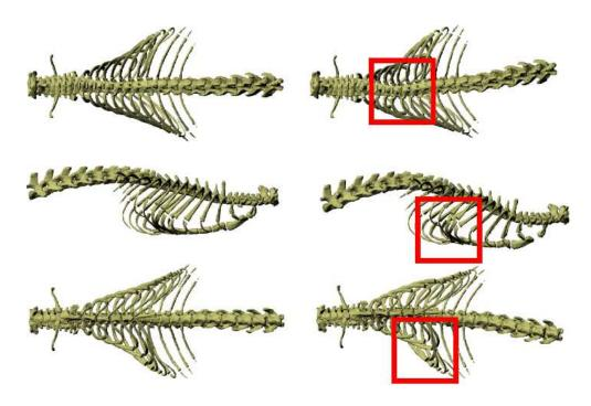
**Figure 2.17:** Top, side and bottom view of the spine and ribcage in the rest pose (left). When deforming the spine and ribcage using only 4 solids (right), the ribs separate (bottom), inter-penetrate (middle) and the deformation of the vertebrae is not smooth (top).
