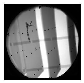
Figure 2.30: Calibration object used for bi-planar X-ray sequences.
