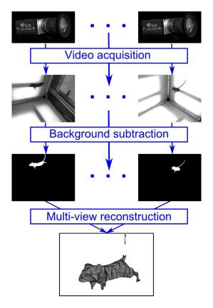
Figure 3.11: Video processing pipeline.
