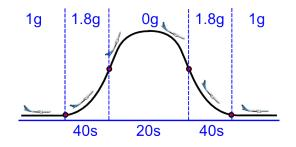
**Figure 1.3:** Simplified profile of the parabola described by the plane during a zerogravity flight. After a period at 1.8 times the gravity (1.8g), micro-gravity (0g) is achieved for about 20 seconds before a new period at 1.8g starts.
