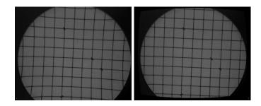
**Figure 1.7:** *Image with distorsion (left) and same image after calculation of the distorsion coefficients and distortion correction.*
