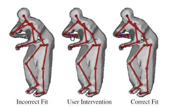
**Figure 4.1:** User intervention when the skeleton is incorrectly fitted to the silhouettes in [VBMP08].
