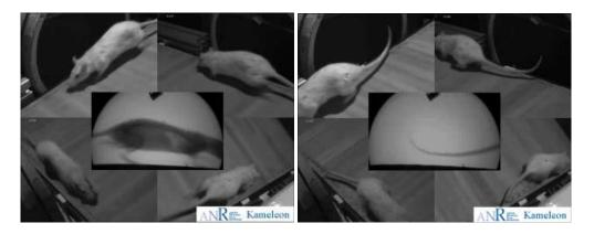
**Figure 1.6:** Set-up for the study of locomotion of rodents. The animal walks on a treadmill in front of an image intensifier (X-rays) and 4 to 6 standard cameras. The lack of constraints of the environment leads to periods of time where the animal is not completely covered (right).
