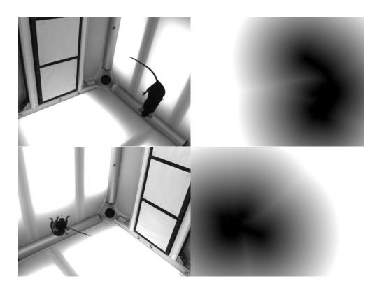
**Figure 4.21:** *Examples for two images (left) of the distance to the silhouette : the darker the pixel, the closest to the silhouette the pixel is (right).*
