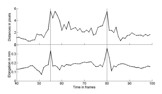
**Figure 2.33:** Diagnosis of errors in the tracking of markers - top row : sum of the distances between the tracked 2D points and the epipolar lines for the markers attached to the radius, bottom row : elongation created by the markers on the radius.
