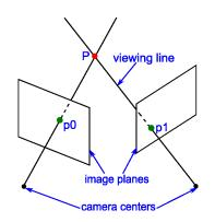
**Figure 2.10:** Triangulation : if the projection of a 3D point P is known in two viewpoints : p0 and p1, then the position of P can be built as the intersection of the 2 viewing lines.
