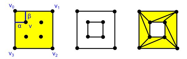
**Figure 3.27:** To create a branch, in case of an extrusion or a fork, first vertices are defined on the quad where the branch is created (left) in order to create a hole (center) then the face is re-meshed around the hole (right).
