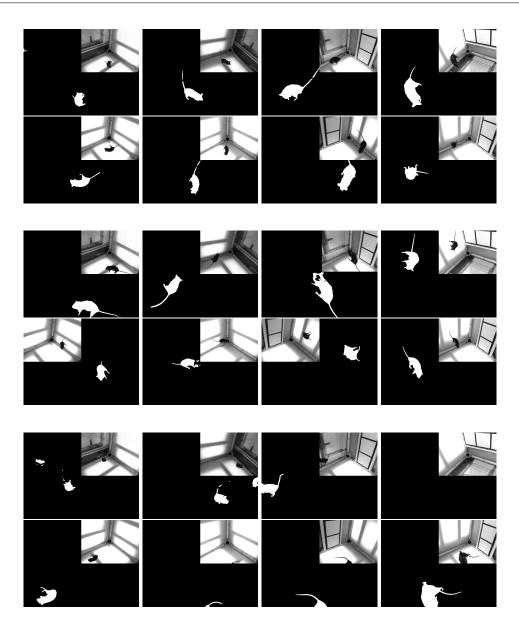
**Figure 3.14:** Examples of background subtraction with the original image on the top right corner : top row shows a case where the results are satisfactory - middle row shows a case where the dark objective of the camera leads to false negative (see the head on camera 3 and 6) - bottom row shows a case where the absence of anti-reflexive material on the top panel leads to false positives (top left on camera 1). The backgrounds are those shown on Figure 3.13.
