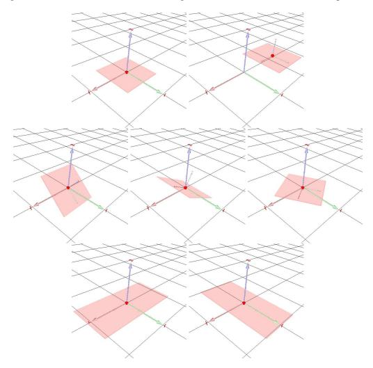
**Figure 3.24:** Different degrees of freedom of an oriented quad - Top row : canonical quad and canonical quad translated - Middle row : rotation about the two directions defined by the quad and rotation about the normal - Bottom row : scale along the two directions defined by the quad.
