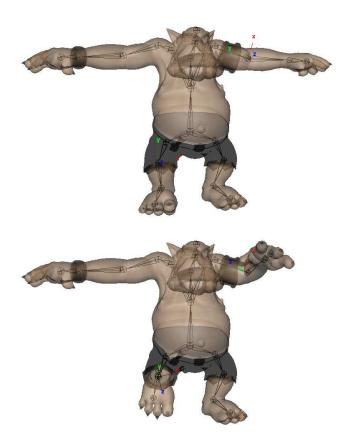
**Figure 3.6:** *Mesh skinned on an animation skeleton : (top) rest pose - (bottom) animation of the left elbow joint and right knee joint.*
