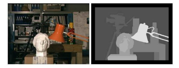
Figure 3.2: Disparity map - left : original image - right : disparity map from [SS02].
