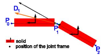
**Figure 2.20:** Illustration of how the control points and tangents of the Hermite spline are computed from the set of articulated solids.
