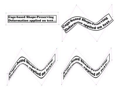
**Figure 3.10:** Deformation of the text top left using Green coordinates (top right), mean-value coordinates (bottom left) and harmonic coordinates (bottom right). Notice how the text is better preserved using Green coordinates [*LLCO08b*].
