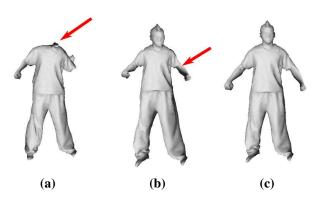
**Figure 4.7:** With the same target model and initial pose as in Figure 4.6 - (a) Result of the optimisation in the oriented quad space. Notice how the head collapses - (b) Result of the optimisation in the 10-D latent space without any regularisation term. Notice how the arms shorten - (c) Result with the regularisation term.
