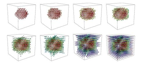
**Figure 1.12:** *Representation of points within the free-floating space that are covered by at least (from left to right)* 8, 7, 6, 5, 4, 3, 2 and 1 camera.
