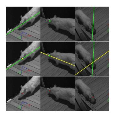
**Figure 2.12:** Example of marker tracking - top row : a point is marked on one camera (green point), the epipolar lines can be computed for the other viewpoints (green lines) - middle row : the same point is marked on another camera (yellow point), it lies on the green epipolar line. The epipolar lines can be computed for the other viewpoints (yellow line) - bottom row : from those two projections, the 3D coordinates of the marker can be computed and projected back to the cameras (red points).
