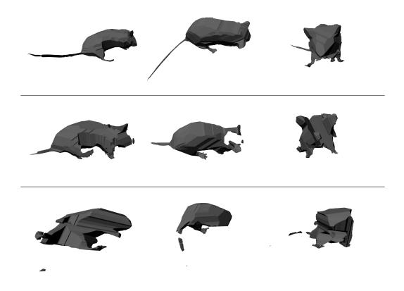
**Figure 3.17:** *Profile, top and front view of the Exact Polyhedron Visual Hulls (EPVH) reconstructed from the silhouettes on Figure 3.14. The quality of the visual hulls deteriorates with the quality of the silhouettes and the number of cameras that cover the mouse.*
