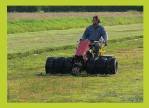
**Figure 32.** Single-axle mower with cutter bar being used to control the common rush.
