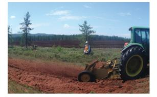
**Figure 22.** Shredding plant material with a rotary tiller, in an undisturbed peatland.
