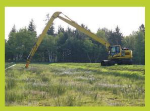
**Figure 33.** Long-reach excavator, equipped with a weed cutter, working from the embankment.
