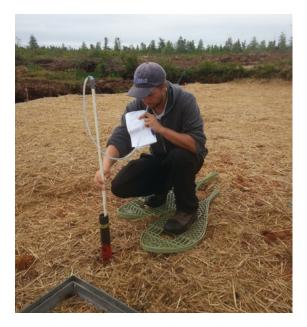
**Figure 29.** A bubbler is used to assess the water level in a hydrological observation well. The bubbler has two parts: a graduated PCV pipe and a flexible tube. Blowing into the bubbler determines the water level, which is measured on the graduated pipe.
