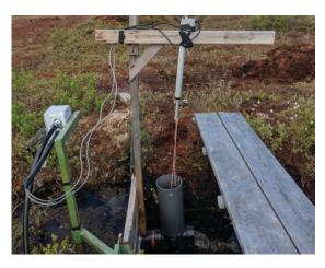
**Figure 19.** Mobile dam operating with a sonar that measures the water level in the reservoir canal, and with a linear actuator and a float (in the grey pipe) to open the dam valve.
