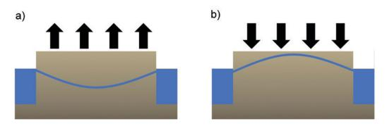
**Figure 17.** Behaviour of the water table in the basins, according to weather conditions: a) In periods of artificial irrigation, the canals have an irrigation effect and the water table is lower as it gets farther away from the canals; b) During times of precipitation, the canals have a drainage effect and the water table is higher as it gets farther away from the canals.
