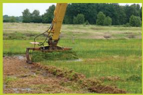
**Figure 37.** Excavator with a weed cutter at the end of its boom being used to cut *Sphagnum*.
