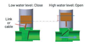
**Figure 18.** Operation of mobile dams. The dam valve is naturally closed and can open via either the linear actuator or float, when the water level is too high in the reservoir canal (illustration taken from the MSc thesis of Guillaume Goulet, 2019).
