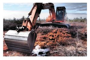
**Figure 21.** Harvesting plant material in a former block extraction site using an excavator with a bucket to scrape the thawed surface layer of *Sphagnum* in spring.
