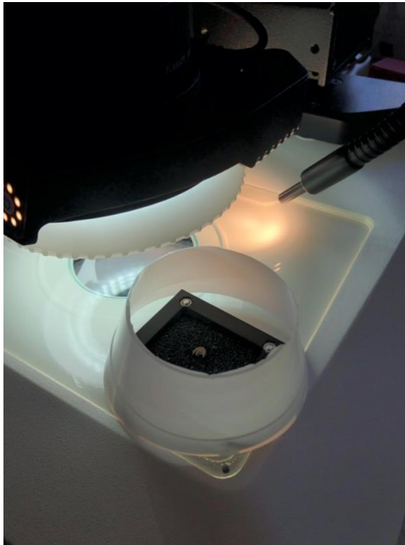
Figure 16. The use of a small plastic dome around the sample to reduce light reflection was not efficient enough.
