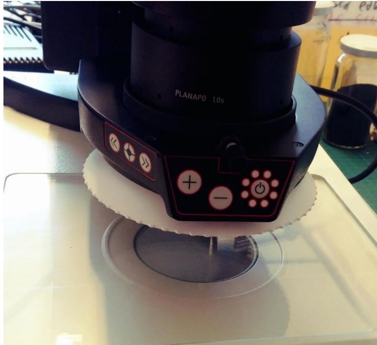
Figure 14. A Leica LED3000 compact LED ring illuminator was used in cases when a bright and homogenous illumination of specimens was needed (also visible in Fig.15).
