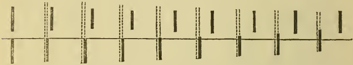
Vernier Diffraction Lines (dotted) seen in Nobert's Plate more or less close to the true.
