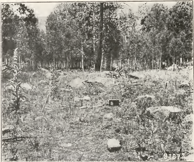
Fig. 1. A typical opening in an aspen stand. A Piche evaporimeter, anemometer, and thermograph are shown in the foreground.
