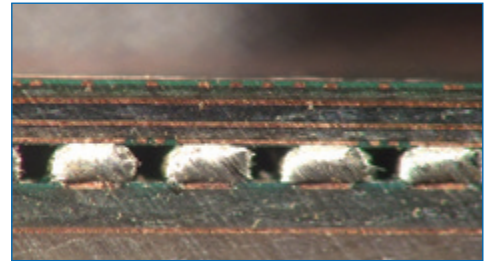
FIGURE 1. The BGA solder balls compressed during reflow. A modified reflow process might be needed.
