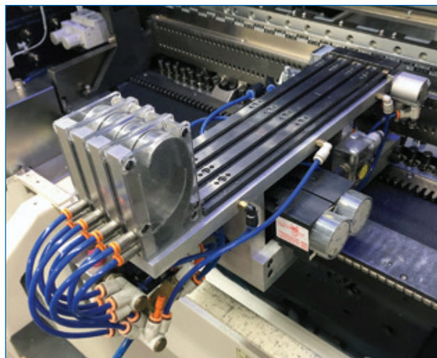
FIGURE 2. To cost-effectively assemble a PCBA with 18 different through-hole socket pins, EDM created a custom odd-form part feeder that utilizes vacuum and compressed air to place the pins during SMT topside placement.
