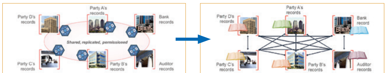
FIGURE 2. Before and after: On the left, a traditional multiparty process consists of multiple two-way exchanges; on the right, the blockchain process permits all parties to access (portions of) the same transaction data.
