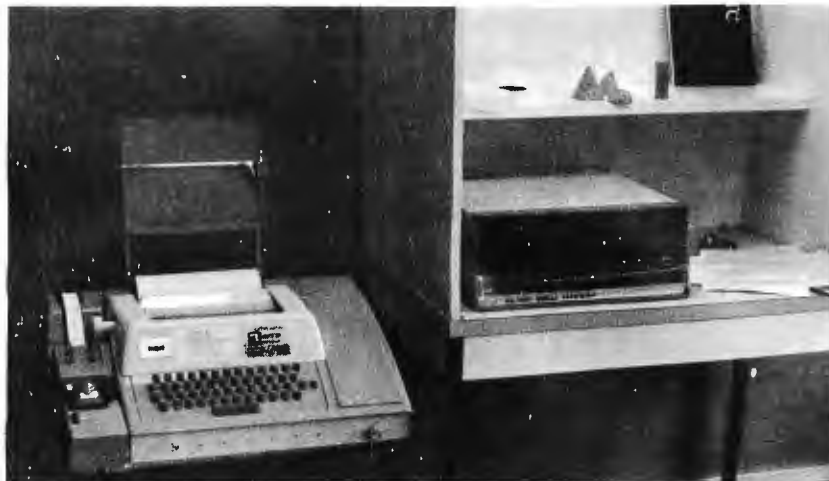
Photo 1: The John F Kennedy High School computing system. There's a Plexiglas shield over the bottom row of switches on the Altair.
