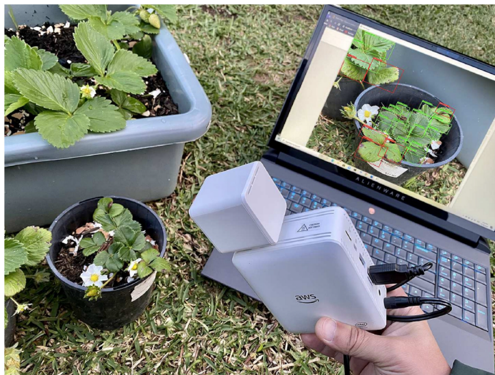
Figure 4.2: Identification & classification of strawberry plant leaf disease by AWS DeepLens in real-time.
